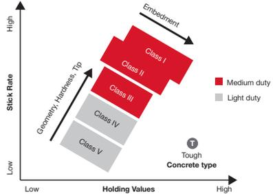
Stick rate of nail classes in different concrete types
