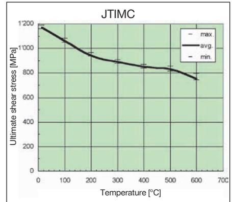
In Japan, similar tests were carried out by JTICM (Japan). These tests were done by driving a 4.5 mm diameter X-CR nail through a 6 mm steel plate into a second 6 mm thick steel plate and shearing the two plates. From the graph it is apparent that the results are nearly the same.
